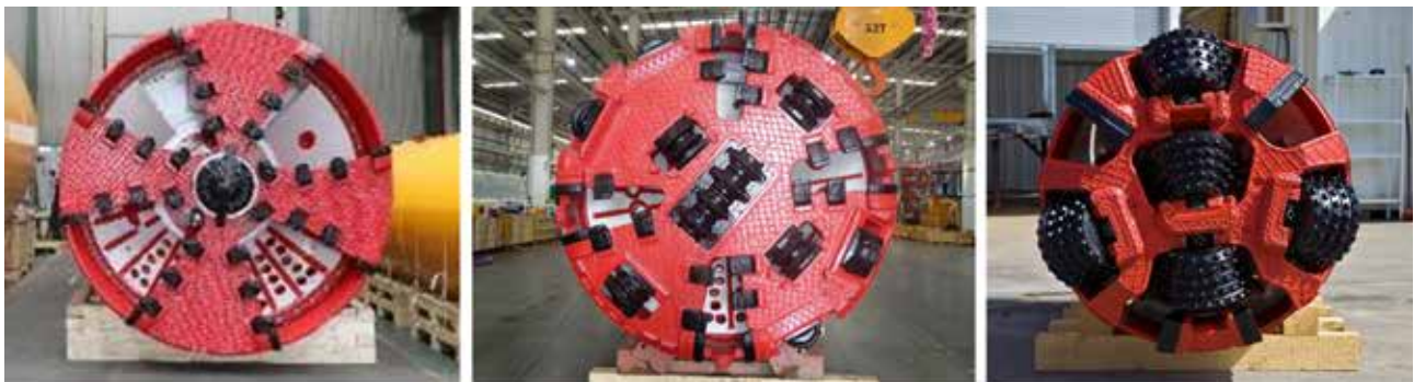
Figure 3. Different AVN cutting wheel designs for soft soil, mixed ground and hard rock (from left right)
