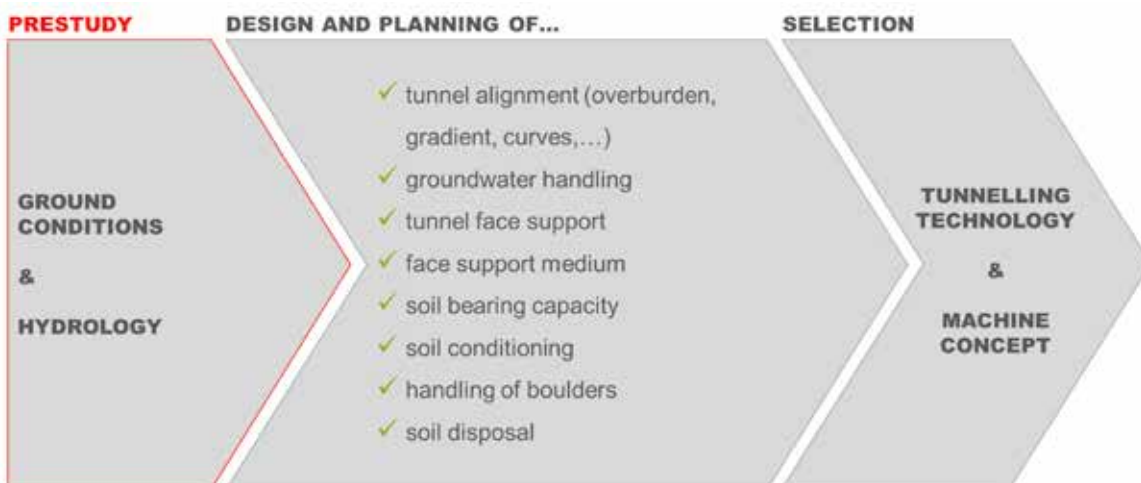
Figure 1. Impact of ground conditions and hydrology on machine selection
