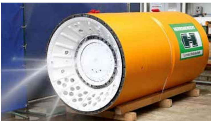
Figure 5. Different jet systems avoid clogging of the crusher cone in cohesive soils
