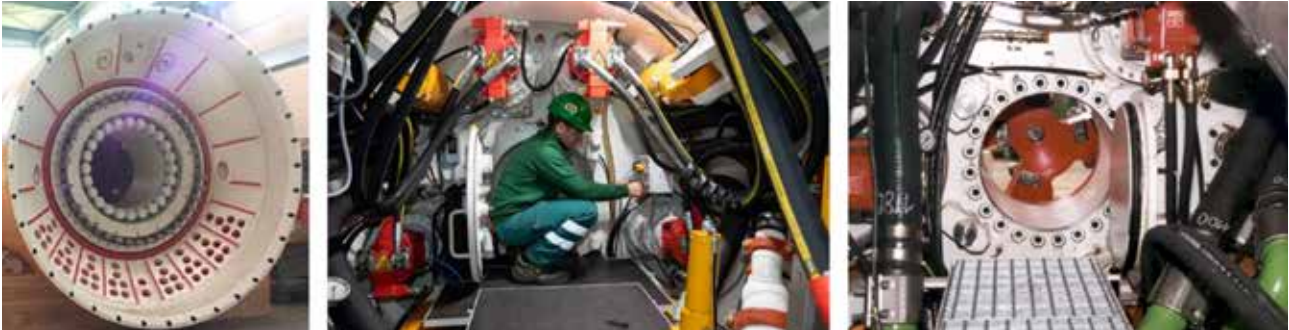
Figure 6. Different jet systems avoid clogging of the crusher cone in cohesive soils
